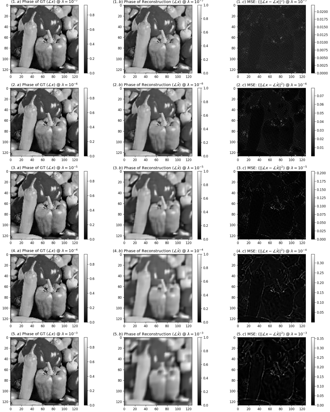
Figure 12: Ground truth (GT) images (a), reconstructed images (b), and corresponding loss results (c) for \lambda = \{10^{-3}, 10^{-4}, 10^{-5}, 10^{-6}, 10^{-7}\} .
